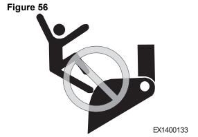
Before lowering any equipment with engine stopped, clear area around equipment of all personnel and bystanders. This procedure will cause high-pressure air or hydraulic pressure to be released to lower equipment.
