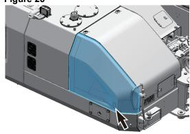
3. Remove mounting bolts (1) and fuel tank cover (2) from frame.
